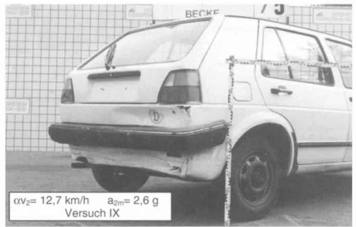
Fig. 10 Comparison of vehicle damages with different degrees of overlap
