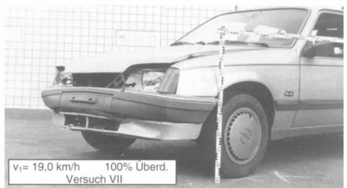
Fig. 10 Comparison of vehicle damages with different degrees of overlap
