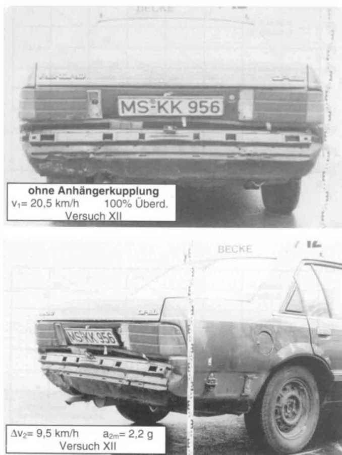
Fig. 14 Vehicle damages with or without trailer coupling
